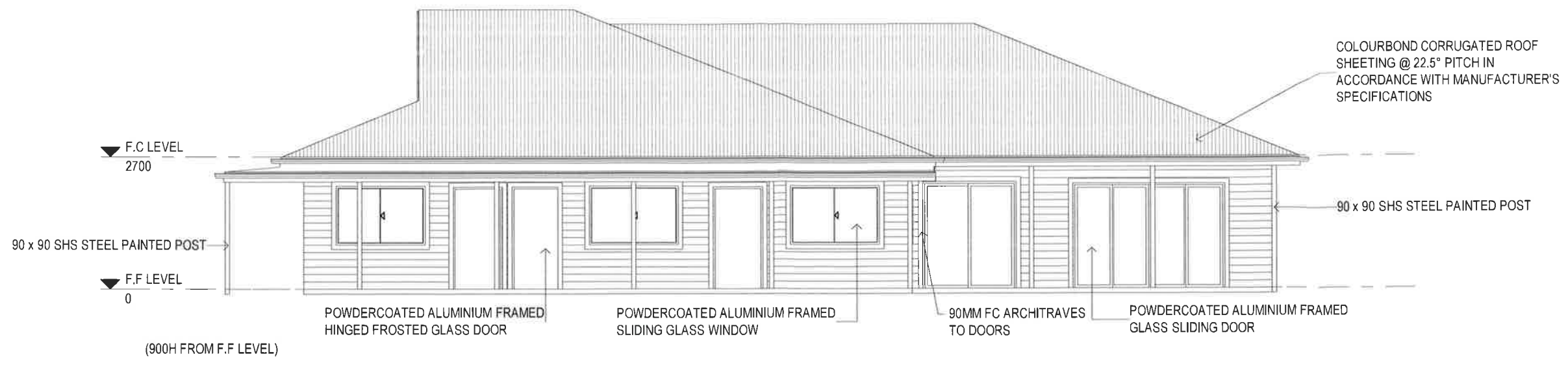
1 OFFICE - EAST ELEVATION 1 : 100
