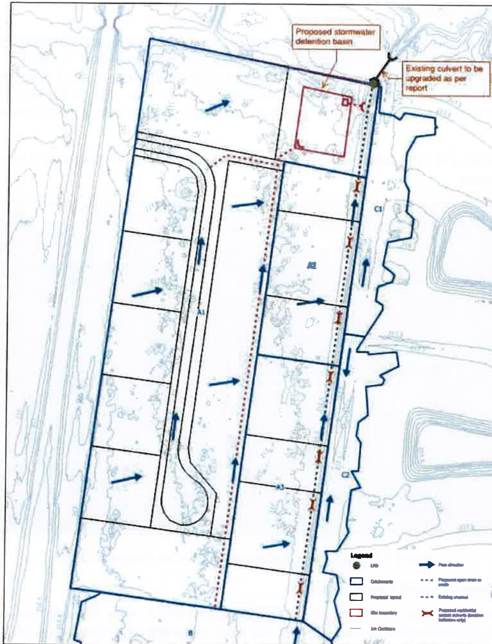
Figure 6.1 Post-Development Drainage Schematic
