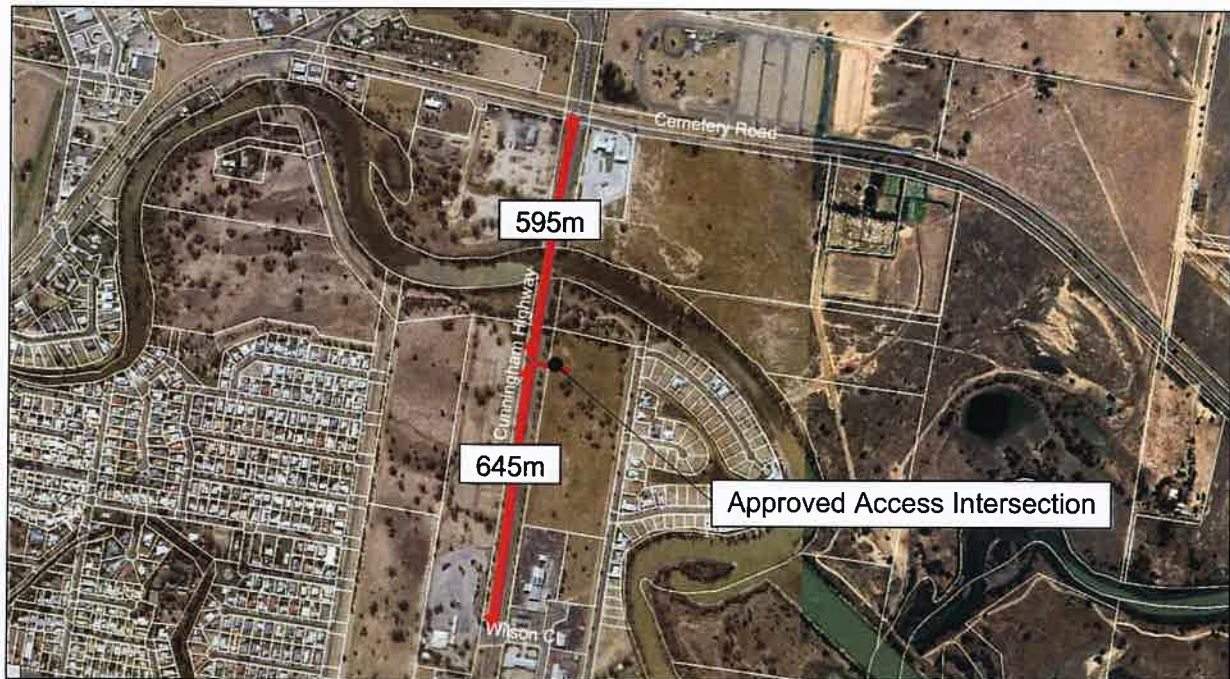
Figure 2.4 Cunningham Highway Intersection Spacing
